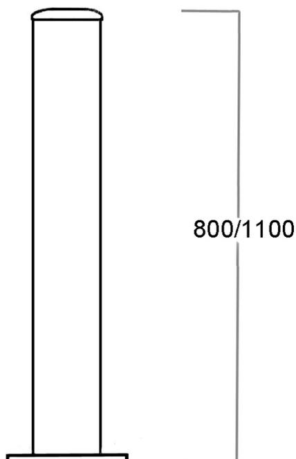
The Civic Bollard provides a functional barrier anywhere that vehicle access restrictions are needed.
